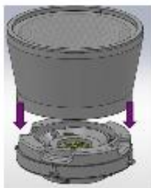
The optic is placed in the groove on the module
