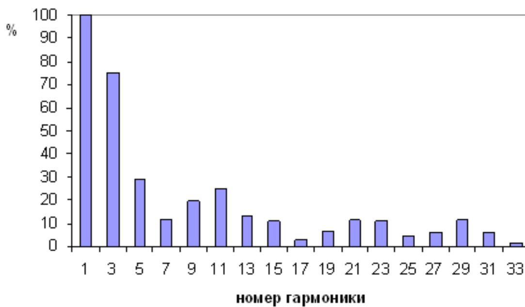
Fig.3. Harmonic composition of the current curve of the lighting units like SDR-27 without PDM( K_{HC}=91,9\% )
